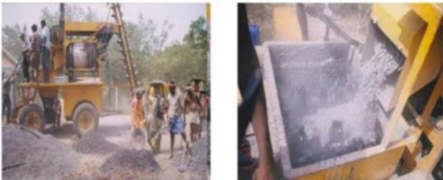
Figure: Mini Hot Mix Plant
