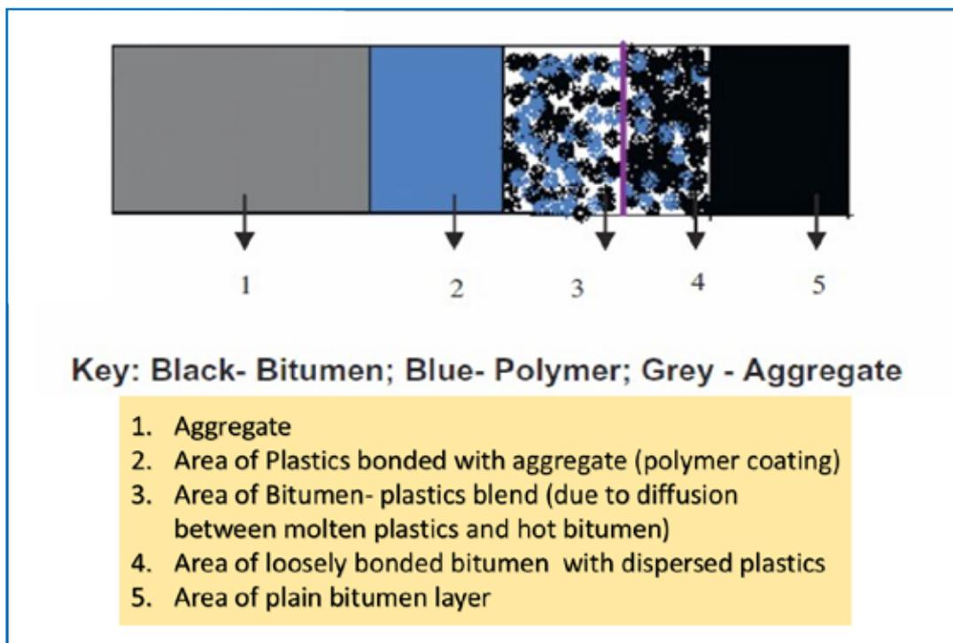
Figure: Bitumen and Plastic Aggregate
