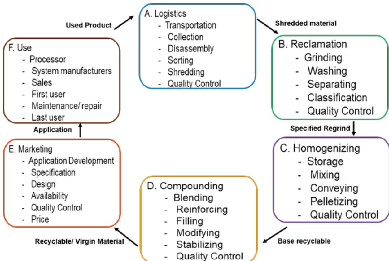
Figure: Mechanical Recycling
