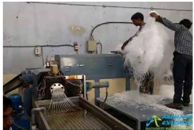
Figure: Extrusion and Palletisation method of plastic waste recycling
