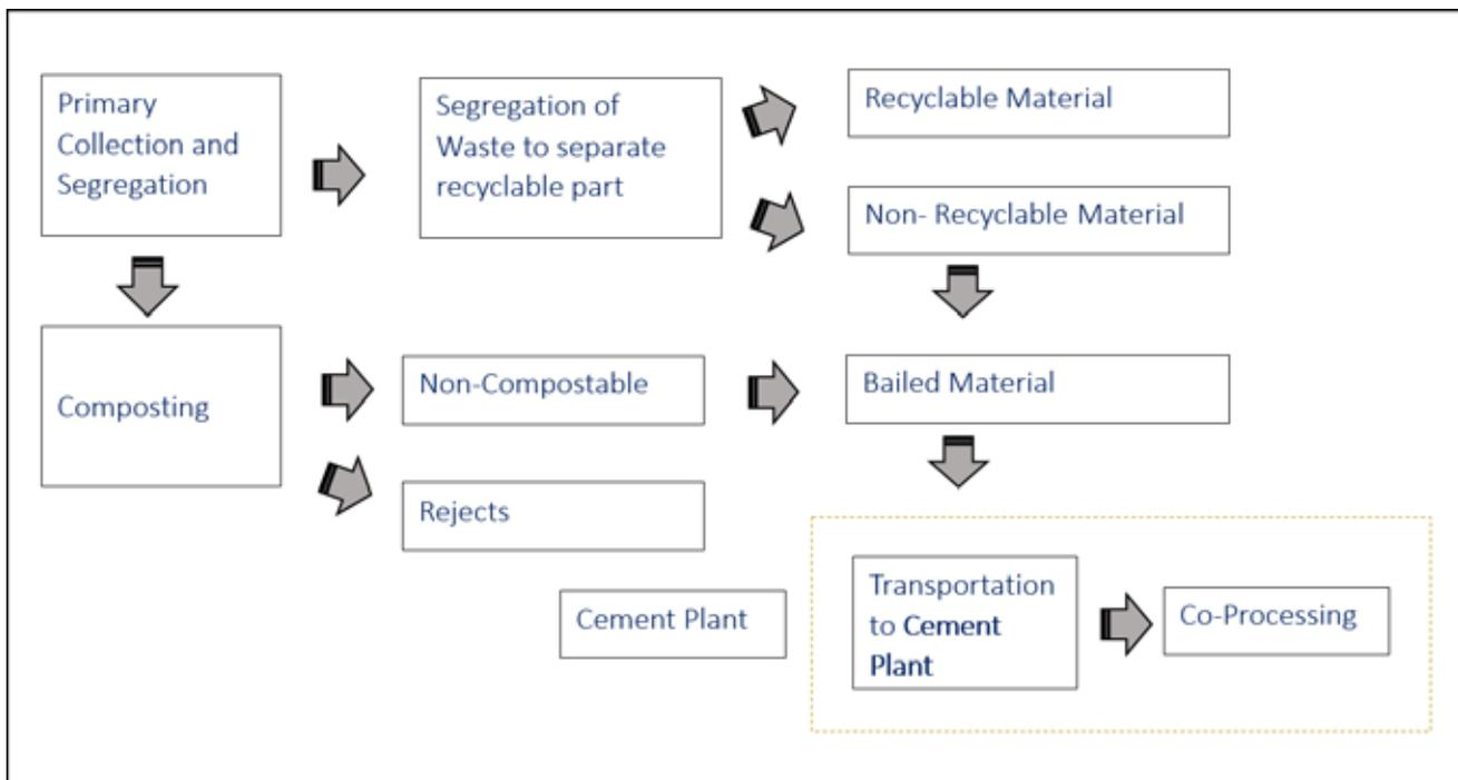
Figure: Co-Processing of Plastic Waste
